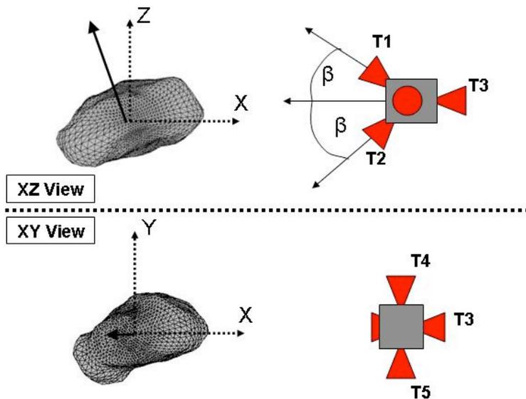
Fig. 2. Diagram of the fixed thruster orientations on the gravity tractor spacecraft relative to the target asteroid (not to scale).
